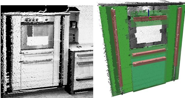
Fig. 5. Region growing based generation of drawer and door hypotheses. *Left*: point cloud data overlaid with reprojected intensity information. *Right*: the same kitchen part overlaid with segmentation results for doors and handles.
